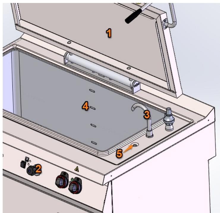
Before starting to boil, it is first necessary to check the water level in the duplicator by opening the overflow tap. If no water is coming out of the duplicator, it is necessary to let the water out by holding the rocker switch. When water starts to flow, close the overflow tap. Note: For AWF versions, skip this step.
